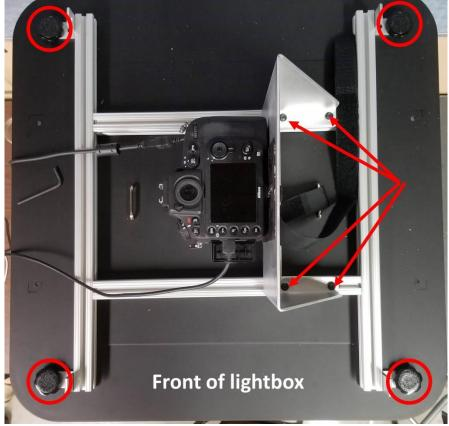
**Figure 5.1** Top view of lightbox with installed camera mount. The knobs that secure the mount to the lightbox are circled in red, and the arrows indicate screws that can be tightened or loosened with a 4 mm Allen wrench to move the camera left or right.
