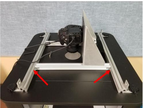
**Figure 5.2** Angled view of top of lightbox with installed camera mount. The arrows indicate screws that can be tightened or loosened with a 2.5 mm Allen wrench to move the camera away from or toward the door of the lightbox.
